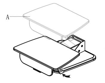
Step 2. Raise the unit by holding the release paddle and lifting the worksurface (A) with both hands. Raise until the arm is sitting at a 45° angle from the base.
