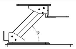
Step 4: Ensuring the arm is still sitting at a 45° angle of the base, insert the largest Allen key into the Tension Adjustment Screw, found at the back of the unit.
